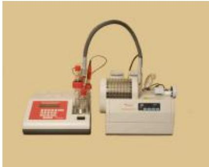
**Evaporators for Oil , Viscuous or Solid Samples
