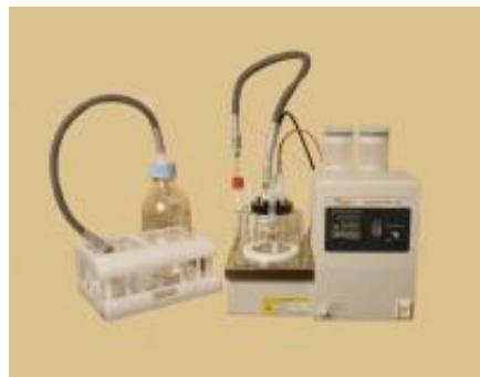
The **ADP 513** Moisture Evaporator can be combined with the**Aquamax** KF coulometric Karl Fischer titrator for water content determination of heavy oils, greases and lube oils which contain additives that interfere with the KF reagents.
