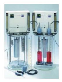
The instrument performs two tests at 24°C and two tests at 93.5°C.
