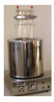
Cleans up to 6 Viscometer tubes at a time (Cannon, Fenske, Ubbelohde, Zeitfuchs and others)
