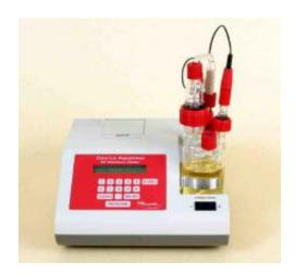
The Coulo Aquamax combines Karl Fischer titration with coulometry to provide fast, accurate, and trouble free water content determination, either in the laboratory or out in the field.
