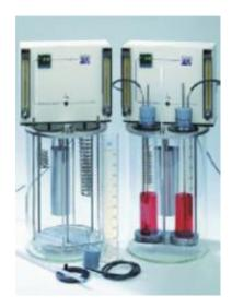
The instrument performs two tests at 24°C and two tests at 93.5°C.
