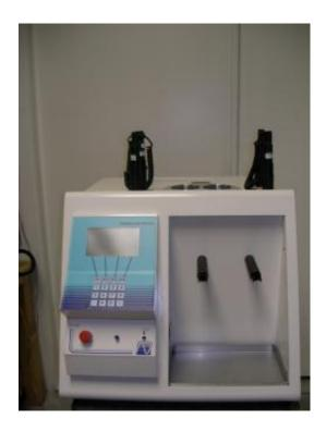
As per ASTM D525, D873, D942, D5304 ISO 7536, IP 40, IP 138, IP 142, NFT 07013
