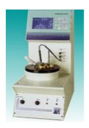
The NTA 440 is delivered with a flame tip detector as well as an automatic gas cutoff at the end of the test process
